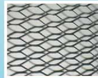
Expanded metal mesh (with different holes) Raw material - HDG and CR Thickness - 0.5 mm Width - 1.0 m Max. length - 9.0 m
